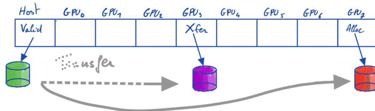
**2x host-to-device transfers (PCIe 3.0 x 16~ 15GB/s) but device-to-device transfer can use high speed network (NVLink DGX1 ~ 96GB/s bi-directional)**
